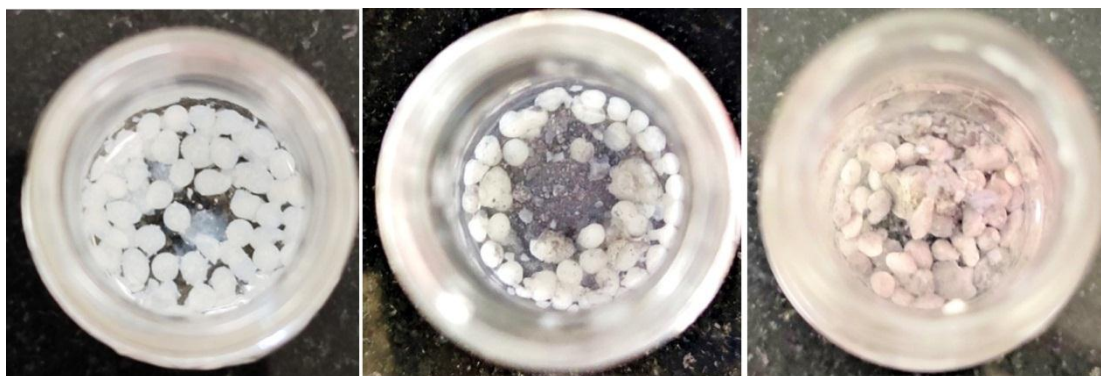
Figure 3.10. Photograph of 22DAP/alginate gel beads from the top of the sample vials showing clear colour change during Ag(I) uptake - (a) without AgNO 3 addition, (b) after AgNO 3 (2 mL of 55 mM AgNO 3 solution) addition after 24 h, and (c) after AgNO 3 (6 mL of 55 mM AgNO 3 solution) addition after 72 h.
