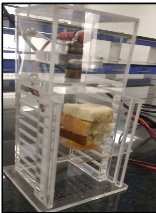
Figure 2. 15: Attenuation coefficient measurement of the food product using GM counter
