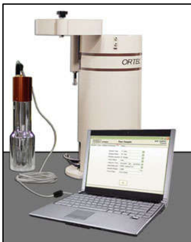
Figure 2. 21: Scintillation Detector for the detection of radiation counts
