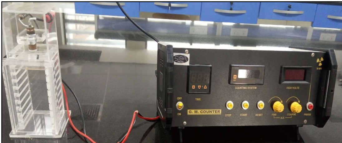
Figure 2. 18: GM Counter to screen the radiation counts.
