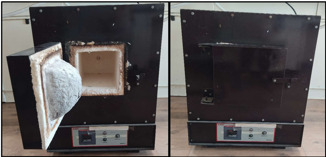
Figure 2. 6: Muffle furnace for the determination of ash
