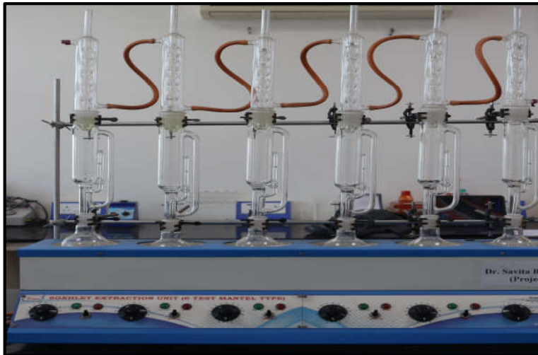
Figure 2. 8: Soxhlet method for fat extraction from food products
