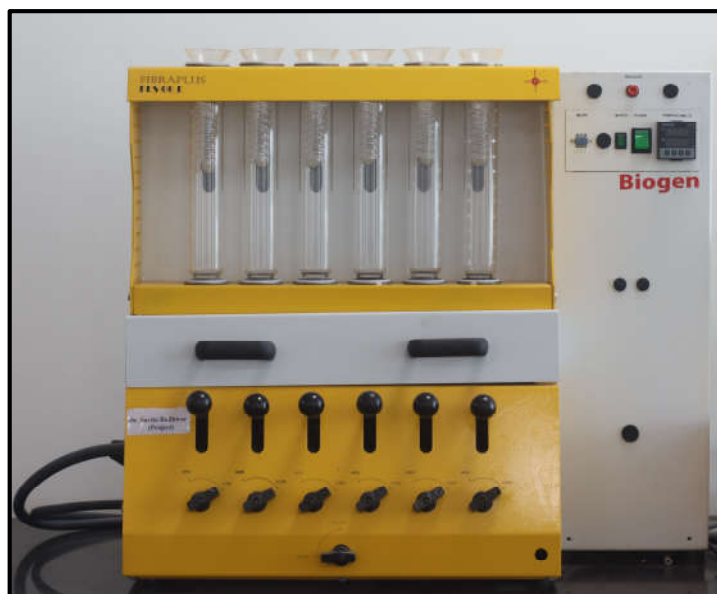
Figure 2. 9: Fibraplus for fibre extraction from food products
