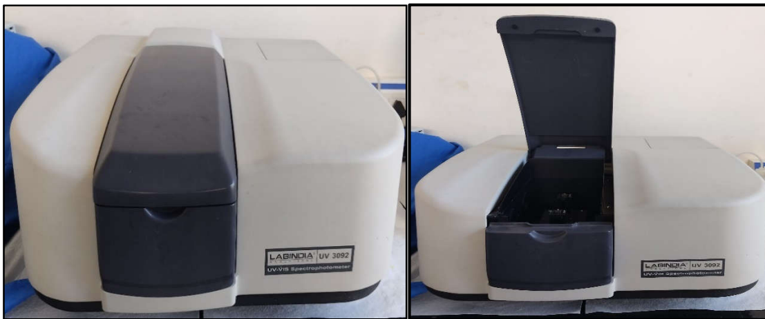
Figure 2. 11: UV-VIS Spectrophotometer for the biochemical estimation
