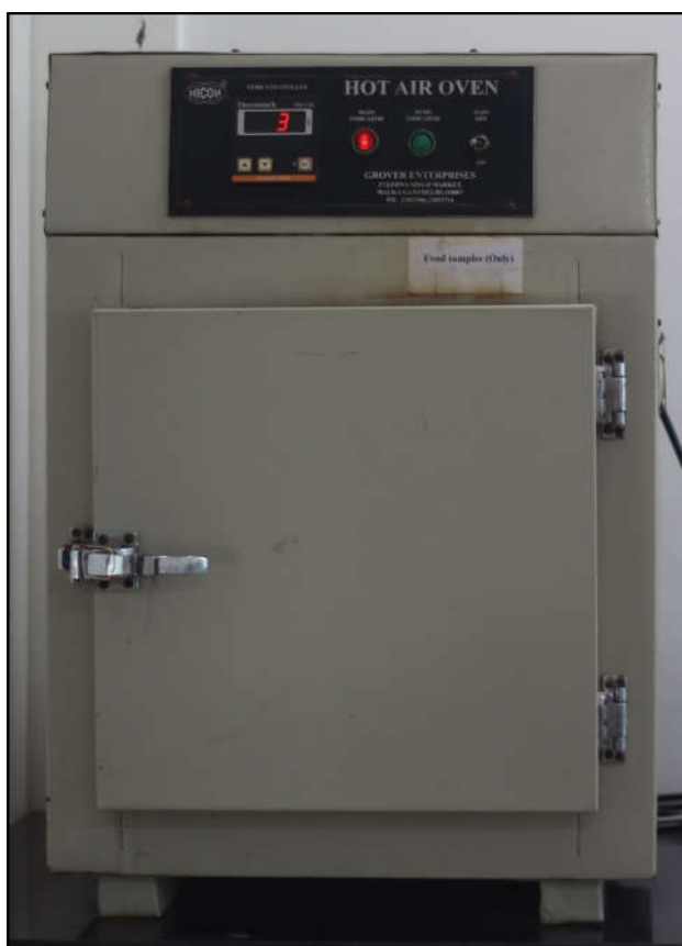
Figure 2. 5: Hot air oven for moisture determination
