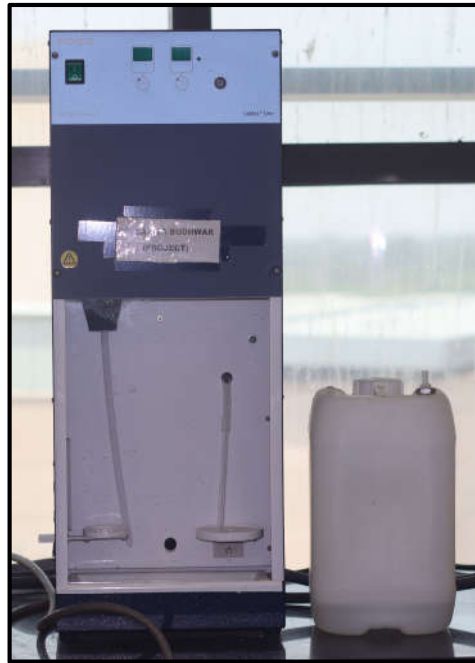
Figure 2. 7: Kjeldahl method for protein estimation using FOSSTM Kjeltec™
