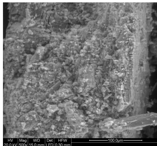
Fig. 13. Cement-mortar mixture containing sand (80%) & wollastonite (20%).
