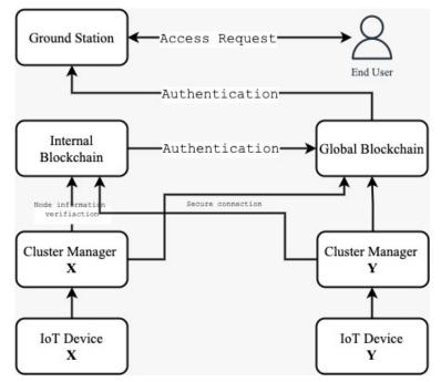
Figure 3. Working framework of proposed mechanism.
