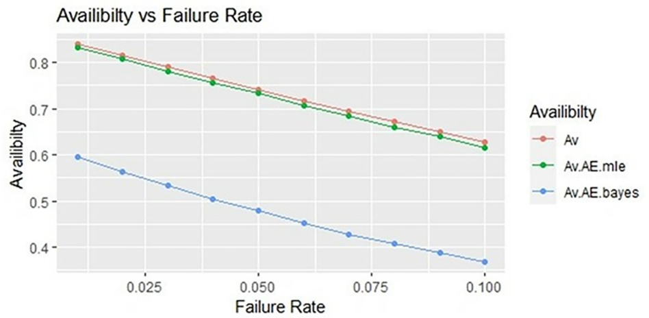
Fig 4. Behaviour of availability with varying failure rate ( \theta_1 ) for \eta = 0.5 .
