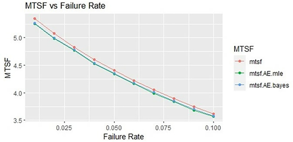
Fig 6. Behaviour of MTSF with varying failure rate ( \theta_1 ) for \eta = 1 .
