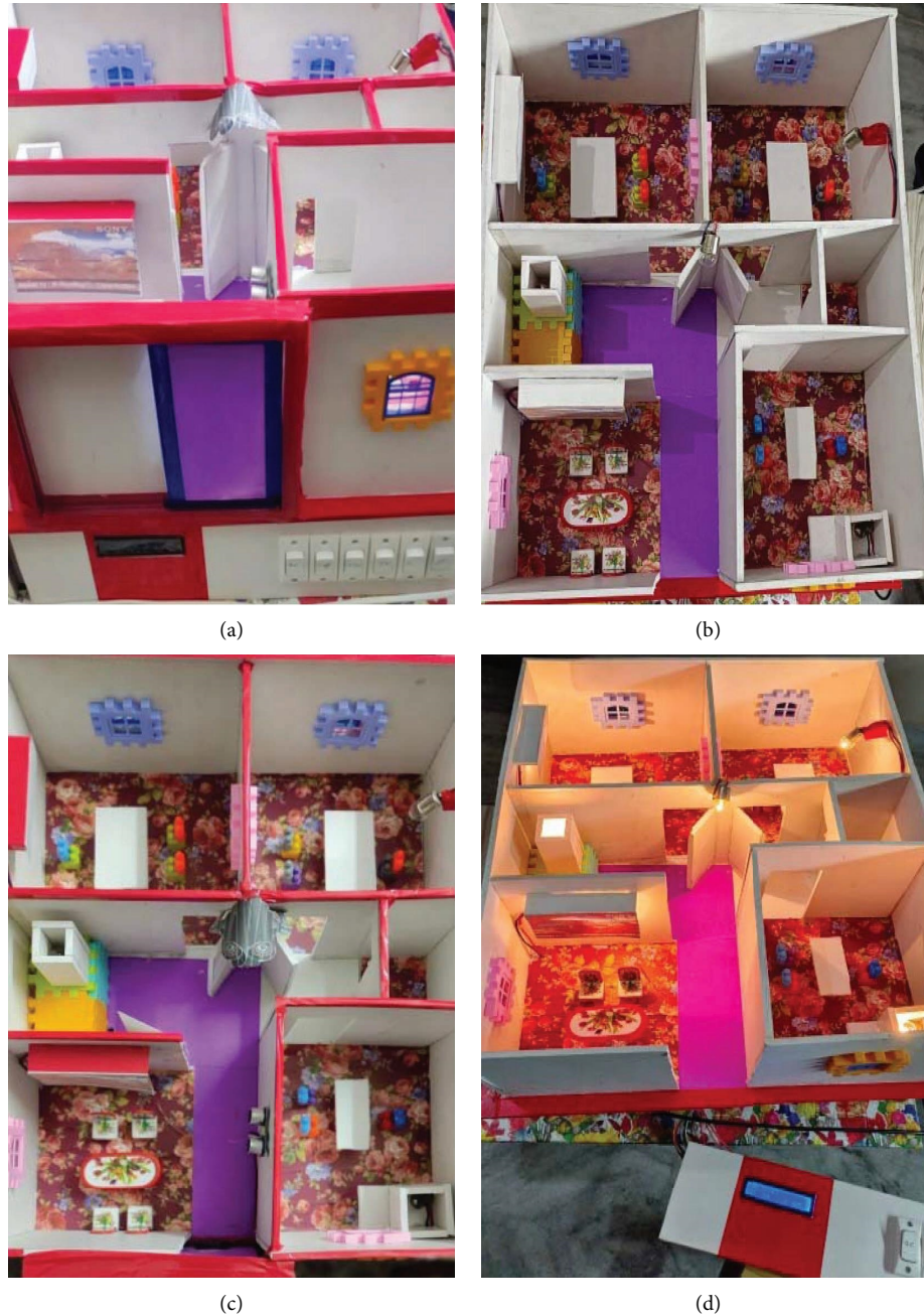
FIGURE 9: Implementation of a smart office prototype. (a) Front view of the initial design. (b) Top view of design. (c) Final prototype with all devices and sensors. (d) Working prototype of the smart office.
